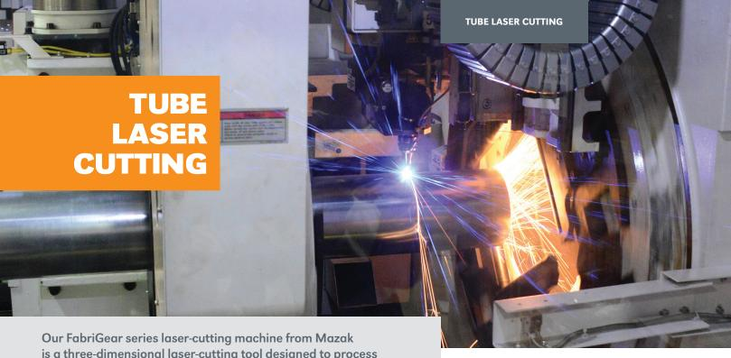
is a three-dimensional laser-cutting tool designed to process a full range of tubes and structures. The machine makes loading raw material into the loading station simple and automatically delivers finished parts to the unloading station. Our tube laser's unique 3D cutting head allows for unsurpassed cutting accuracy at any angle for the best part fit and weld preparation.
